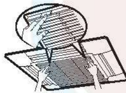
Fig. 6.5: Opening the suction grill
